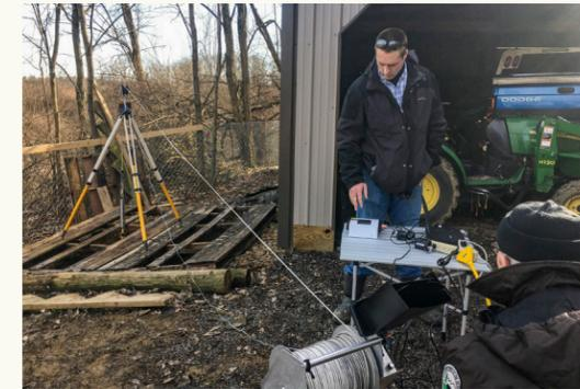
Indiana AML worked with OSMRE to visually analyze the boreholes using a downhole camera.
