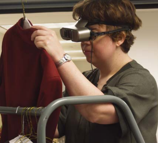
The JORDY (Joint Optical Reflective Display) Magnifier enables this legally blind woman to work through newfound "sight."
