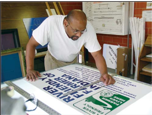
PEN Product offender workers at the Westville Correctional Facility make highway regulatory custom signs for the Indiana Department of Transportation and private customers. New computer-aided design equipment has improved the quality and consistency of the manufactured signs.
