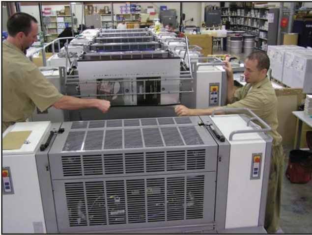
The 6-color press and disk to plate pre-press equipment greatly increased PEN Products printing capabilities.
