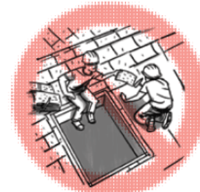
DON'T work around unprotected openings or skylights
