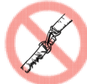
DON'T use defective equipment
