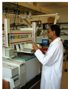
Preparing the GC/MS for Methamphetamine analysis.
