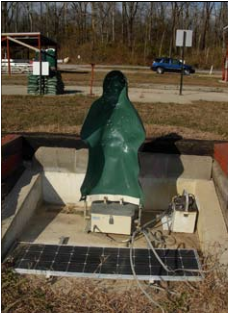
(Above) Note the solar panels on this pop-up target. Since field artillery can happen at any time, batteries are hooked up for use when the power from the solar panel is drained.
